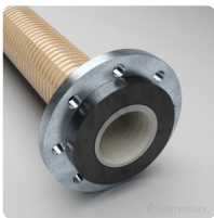
Combiflex Cast-on PU Swivel Flange Fixed cast-on PU loose flange for all Master-PUR hoses, for counterflanges to DIN 2632 / DIN 2633 / DIN 2673
