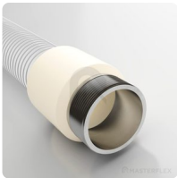
Combiflex VA Threaded Sockets Food cast-on VA threaded socket with male thread to DIN ISO 228 for all Master-PUR Food hoses, food-safe EU 10/2011
